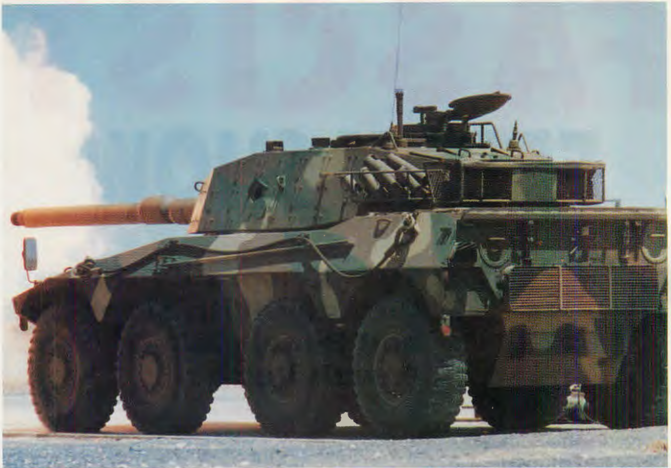
Rooikat 105 Tank Killer fires its GT7 rifled tank gun, which can employ all standard NATO 105mm ammunition.
